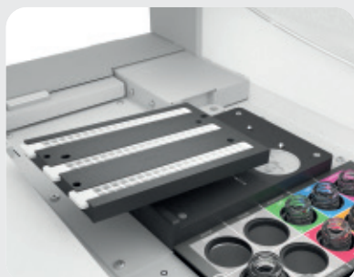
1 V8 UltraCE automatically dilutes samples and loads the sample tray
